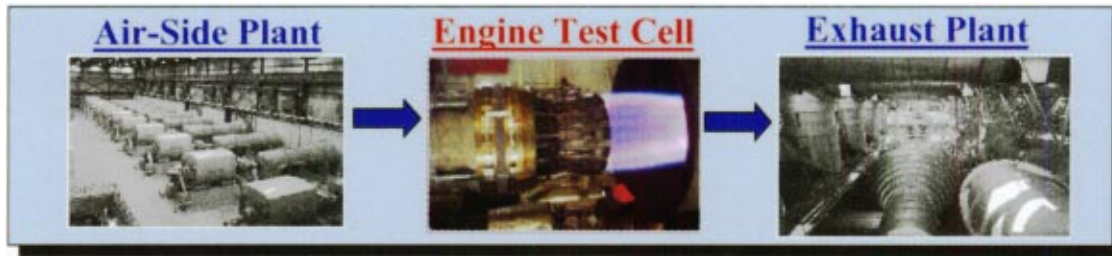
Fig. 1 Typical ground test facility/engine configuration
